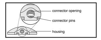
Look inside the transmitter's connector opening to make sure that the connector pins are not damaged or corroded. If the connector pins are damaged or corroded, the transmitter cannot communicate with the charger or pump. Contact the 24 Hour HelpLine or your local representative. It may be time to replace your transmitter.
