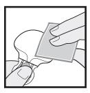
10 Holding the tester, wipe the transmitter with 70% isopropyl alcohol.
