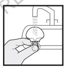
5 Prepare a cleaning solution using one teaspoon (five milliliters) of mild liquid soap per one gallon (3.8 liters) of room temperature tap water. Never use organic solvents, such as paint thinner or acetone, to clean the transmitter.
