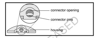
Look inside the transmitter's connector opening to make sure that the connector pins are not damaged or corroded. If the connector pins are damaged or corroded, the transmitter cannot communicate with the charger or pump. Contact the 24 Hour HelpLine. It may be time to replace your transmitter.
