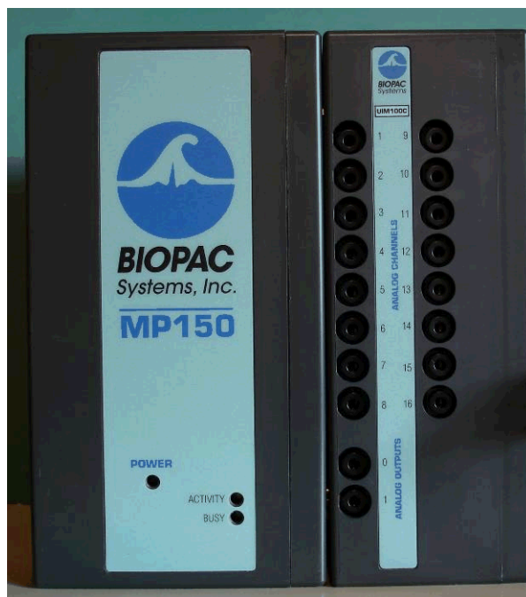
Figure 2. Biopac MP150 Data Acquisition System with Biopac UIM100C Module.
