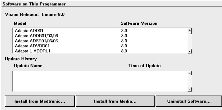
The programmer displays the Software on This Programmer screen and lists the software already installed on the programmer. For each model, the screen displays the software version.
