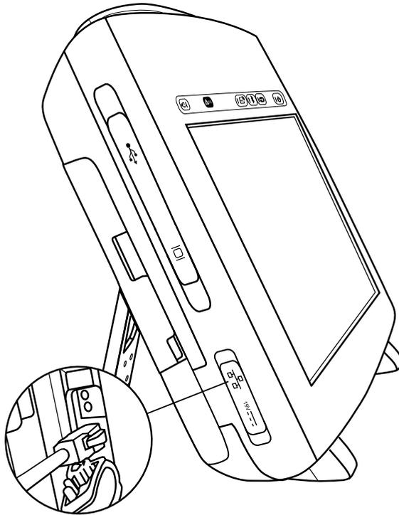
1. Open the input cover on the lower left side of the programmer.
