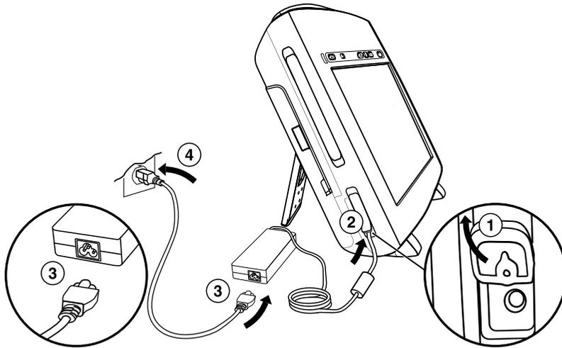
1. Open the power input cover on the lower left side of the programmer.
