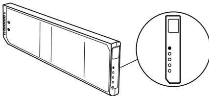
Check the battery charge capacity periodically with the built-in indicator. Replace the battery pack when the battery charge capacity is less than 60% of the original/new charge capacity, and/or when the battery charge time increases significantly.
