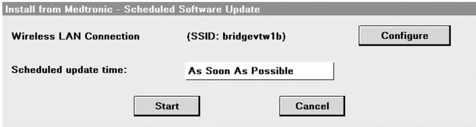
5. On the Scheduled Software Update screen, either choose to start the download at a particular time by selecting a time from the pull-down menu, or begin the download as soon as possible by pressing [Start]. The programmer shuts down and displays a window telling you to please wait.
