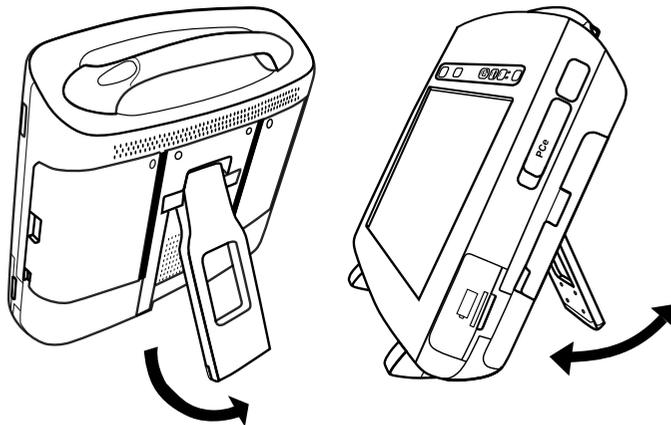
1. To position the programmer at an angle, pull out the stand on the rear of the programmer.
