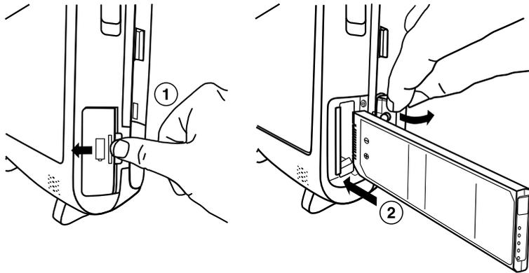
1. Open the battery door on the lower right side of the programmer by pressing forward on the battery door recess and flipping the door to the left.
