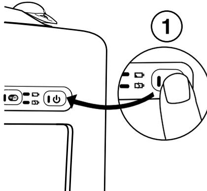
1. Locate the Power button on the front right corner of the programmer button panel.
