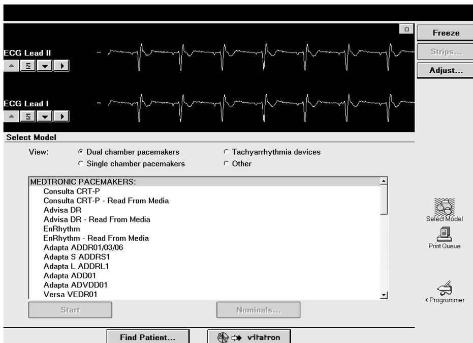
If the Select Model screen does not look like this example and you see a different button in the command bar, press the Vitatron/Medtronic switch button to display this screen.
