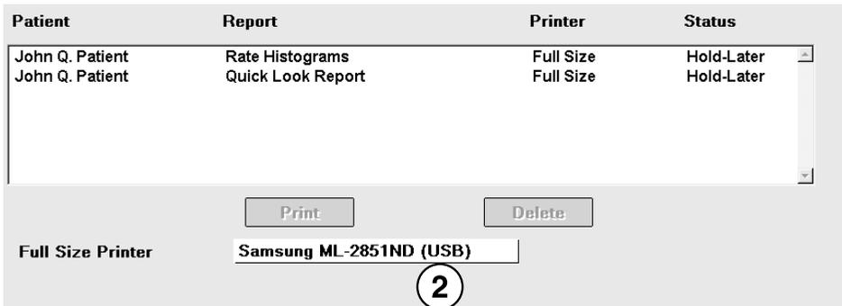
2. On the Print Queue screen, select the Printer field to open the list of supported printers.
