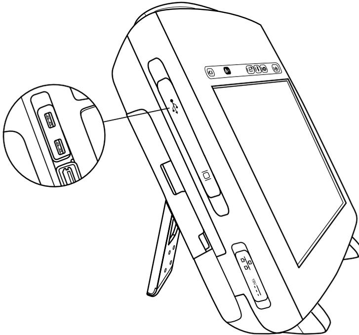
1. To connect to a printer with a USB cable, locate a USB port. There are two USB ports located on the left front side of the programmer.
