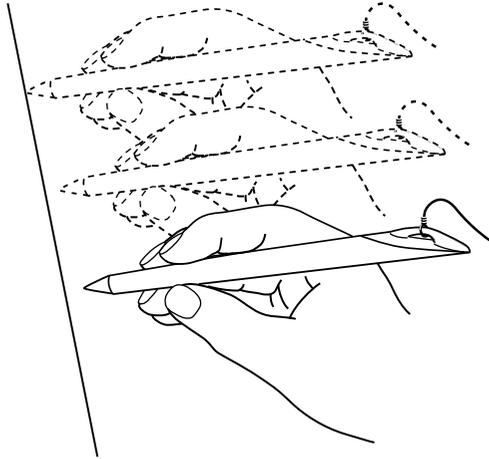
1. Move the tip of the stylus to a position directly over the desired option. If the desired option is a displayed key or button, position the stylus tip within the rectangular outline. If the desired option is a name or number, such as a parameter or parameter value, position the stylus directly over the letters or numbers forming the option.
