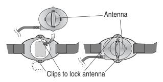
Figure 2.2 Attach the antenna to the belt.
