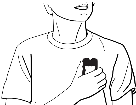
Figure 3. Hold the Patient Assistant in front of the implanted device. (The device may be implanted in a different location than is shown here.)
