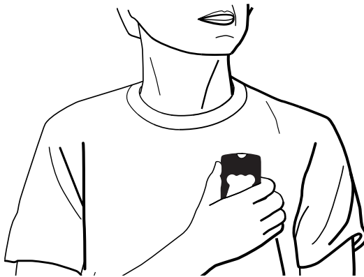
Figure 5. Hold the Patient Assistant in front of the implanted device. (The device may be implanted in a different location than is shown here.)
