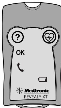
Figure 6. Reveal XT Patient Assistant model 9539 showing all possible response indicators when the Query button is pressed.
