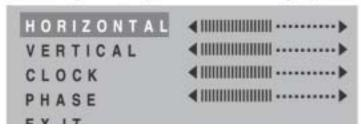
**HORIZONTAL**: Adjusts the horizontal position of the display.
