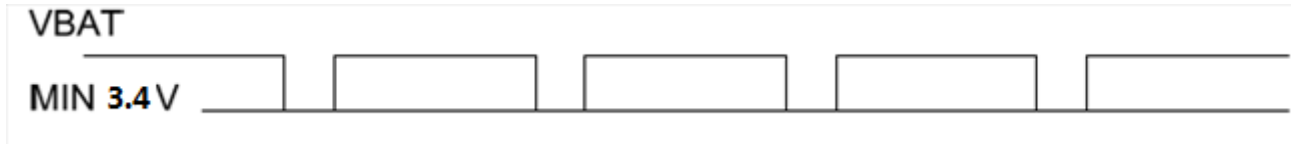
Figure 4.4: VBAT lowest voltage drop
