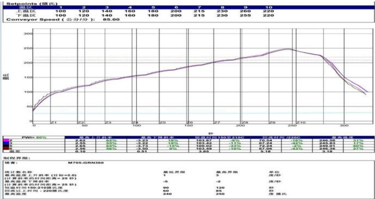
Figure 49: Module recommended soldering furnace temperature curve
