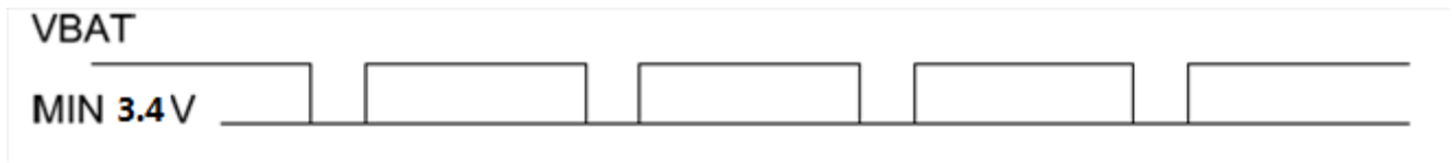
Figure4.4: VBAT lowest voltage drop
