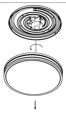
1. Turn the c1asp and remove the 1amp shade downward
