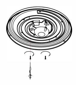
4. Insert the 1amp body through the screw and turn the 1amp body Unti1 the 1amp body cannot be removed through the screw head, then 1ock the screw
