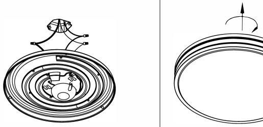
3. Connect the  $b^1$ ack wire of the 1amp with two wires of the same  $co^1$ or on the junction box with the wiring cap provided, and connect the ground wire of the 1amp with the ground wire of the wiring  $go^1$ d.
