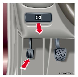
To engage, firmly depress parking brake pedal. When the electronic key is in starter switch position 2, the brake warning lamp in the instrument cluster should come on brightly.
