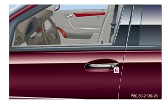
6 Infrared receiver in driver's door handle
