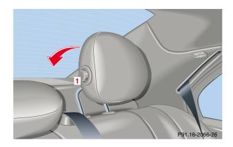
Folding head restraints back in the rear passenger compartment:
