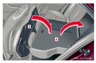
1. Pull backrest (4) up until it locks in its upright position. Check for secure locking by pushing and pulling on the backrest.
