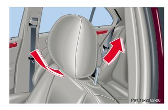
Adjust the head restraint angle by hand. Push or pull the head restraint in direction of arrow.
