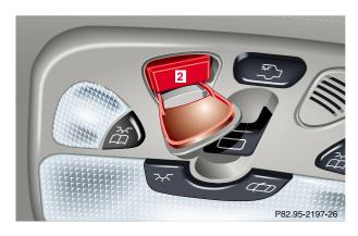
Press the emergency call switch (2) briefly (for longer than 2 seconds). The indicator lamp in the emergency call switch (2) will flash until the emergency call is concluded. Wait for a voice connection to the Response Center.
