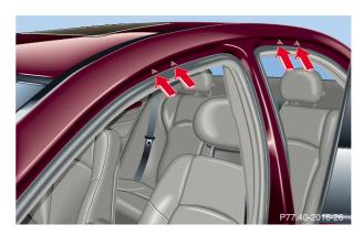
Only mount roof racks to the fastening bolts (see arrows) located under the door weatherstrips.
