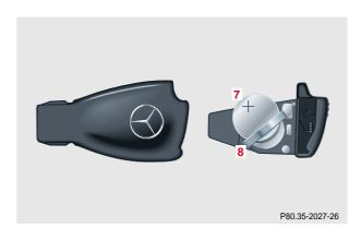
Change batteries (7), inserting new ones under contact spring (8) with plus (+) side facing up.
