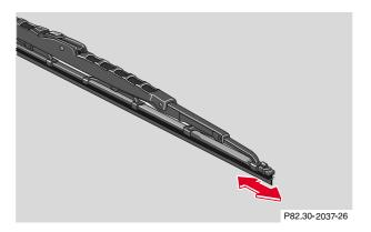
Place wiper blade on firm support. Press down both tabs and slide (direction of arrow) the wiper blade insert out of the retainer claws.
