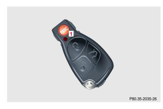
To activate press and hold button (1) for at least one second. An audible alarm and blinking exterior lamps will operate for approximately 3 minutes.
