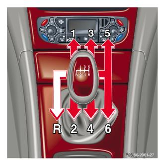
See illustration for gearshift lever positions corresponding to the individual gears.
