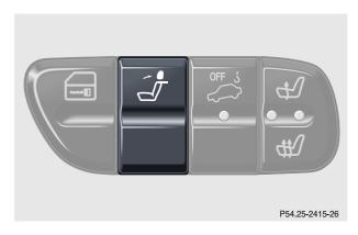
Folding head restraints back with switch in the center console:
