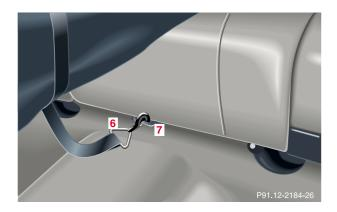
8. Connect snap hook (6) of front strap to eye (7) located on center tunnel in front of rear seat bench.
