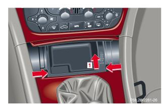
Slide ashtray insert in direction of arrow (1) until the insert disengages. Grip ashtray insert at indents (left and right arrows) and remove from ashtray frame.
