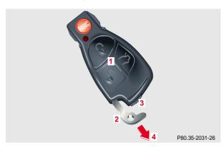
The electronic main key has an integrated radio frequency and infrared remote control, plus removable mechanical key.
