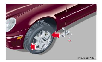
11. Clean contact surfaces of wheel and wheel hub. Install spare wheel on wheel hub. Insert wheel bolts and tighten them slightly.
