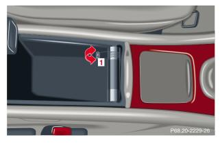
The front center console compartment has its own air outlet.
