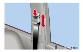
4 Button for belt outlet height adjustment
