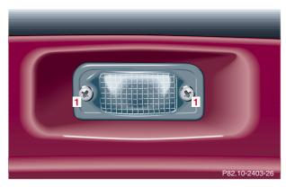
Loosen both securing screws (1), remove lamp and replace tubular lamp (C 5 W/4 cp).
