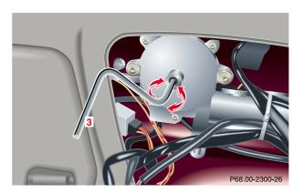
Obtain crank (3) (supplied with vehicle) and insert through hole.
