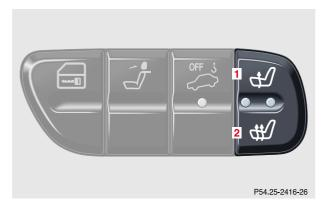
The front seat heaters can be switched on with the electronic key in starter switch position 1 or 2.
