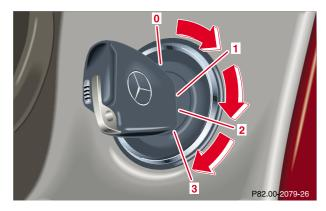
O The electronic key can be withdrawn in this position only. The steering is locked when the electronic key is removed from the starter switch. If necessary, move steering wheel slightly to allow the locking mechanism to engage.
