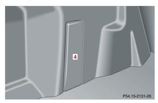
**4** Auxiliary fuse box in left hand side of trunk.
