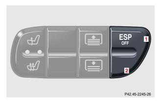
ESP control switch located on center console.
