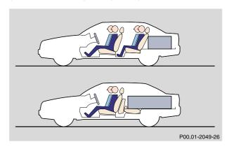
The total load weight including vehicle occupants and luggage/cargo should not exceed the vehicle capacity weight indicated on the certification tag which can be found on the left door pillar.
