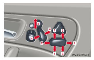
The switches are located in each front door.
