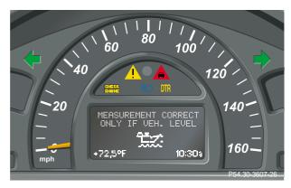
To check the engine oil level, park vehicle on level ground, with engine at normal operational temperature.
