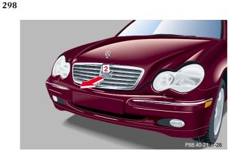
Pull handle (2) to its stop out of radiator grill and open hood (do not pull up on the handle).
