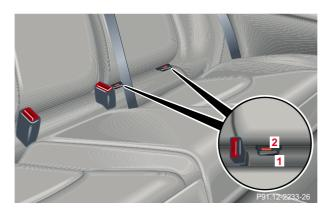
This vehicle is provided with two mounts (at each of the outer rear seats) for the installation of a child seat having the matching mounting fittings. The mounts can be folded back between the seat cushion and the backrest.
