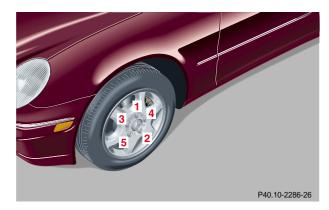
13. Using the wrench, tighten the five bolts evenly, following the sequence illustrated, until all bolts are tight.
