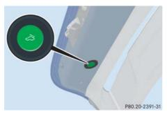
The emergency release button is located in the trunk lid.
