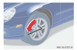
On wheel to be changed, loosen but do not yet remove the wheel bolts (approximately one full turn with wrench).
