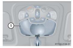
▶ Pry off lens 1 using a screwdriver.
