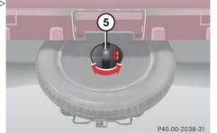
When storing the space-saver spare wheel in its holder, secure it using the bayonet lock.
