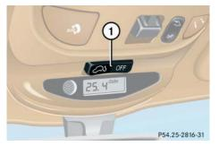
Switching off tow-away alarm and glass breakage sensor
