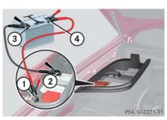
Positive terminal of discharged battery
