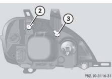
(2) Headlamp vertical adjustment screw(3) Headlamp vertical adjustment screw
