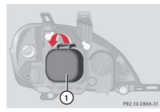
Low beam halogen or Bi-Xenon\* headlamp cover with locking tab
