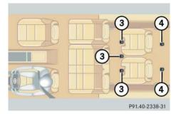
(3) Anchorage rings for second row seats(4) Anchorage rings for third row seats\*
