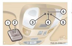
Remote control integrated into the overhead control panel
