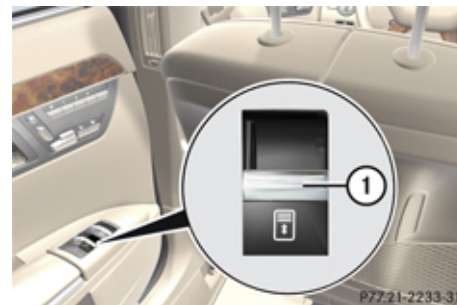
Rear door control panel
