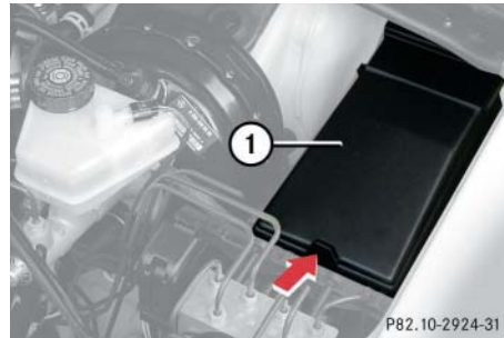
① Main fuse box
