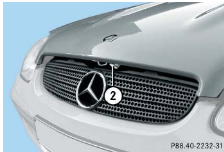
② Lever for opening the hood
