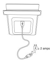
1. Connect the supplied Micro USB cable to the Wireless Charging Stand's input port and then connect it to a USB-A adapter (2 amps or QC 2.0).
