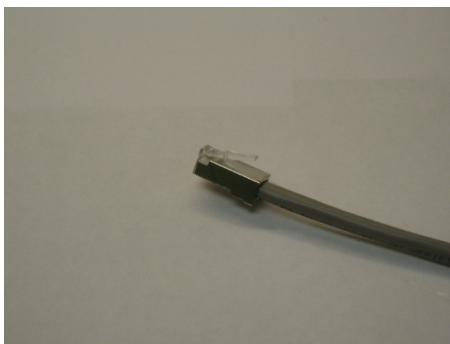
Figure 35 – Cable RJ45 Connector
