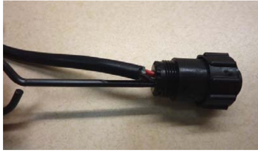
Figure 29: Use insertion tool to secure the pins in the plug.
