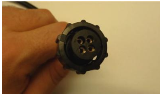
Figure 31: Front view of plug with crimp pins properly inserted
