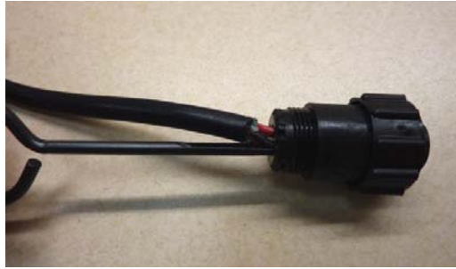
Figure 30: Use insertion tool to secure the pins in the plug.
