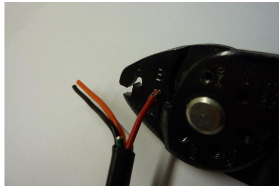
Figure 26: Complete the second crimp with tool section “B”.
