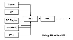
Analogue sources need to be converted to digital before passing through 518. Meridian make the 562 and 562V digital controllers, both of which have very high quality delta-sigma analogue—digital converters.
