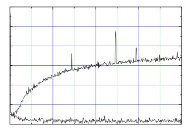
Figure 1. Showing jitter spectrum of twin PLL.
