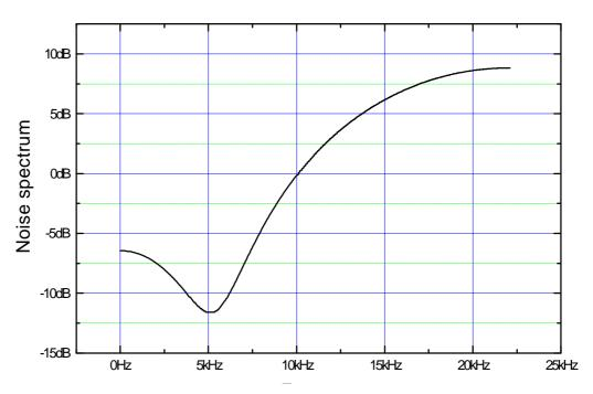
Above: noise spectrum for Shape A at 44.1kHz.
