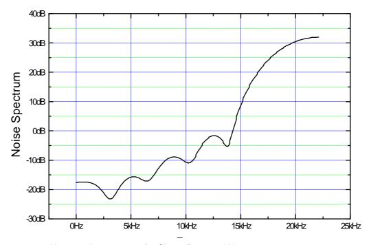
Above: noise spectrum for Shape B at 44.1kHz
