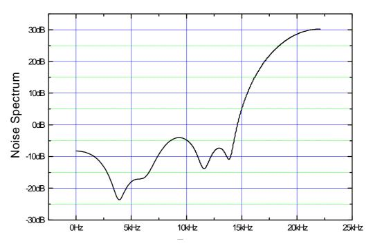
Above: noise spectrum for Shape C at 44.1kHz
