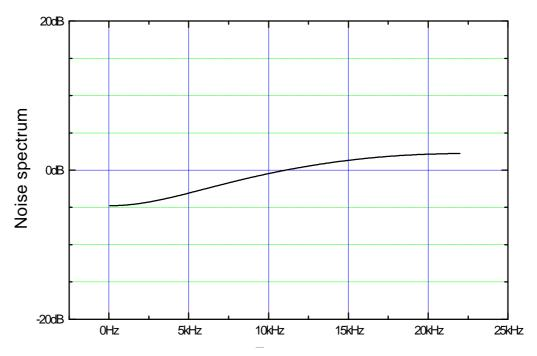
Above: noise spectrum using High-Pass additive TPDF dither at 44.1kHz
