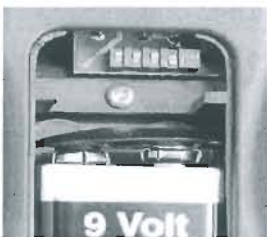
Figure 5: DIP Switch in Remote Handset Battery Compartment
