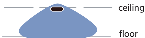
Figure 43: Coverage Pattern for AP332i When Ceiling Mounted
