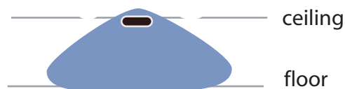
Figure 14: Coverage Pattern for AP320i When Ceiling Mounted
