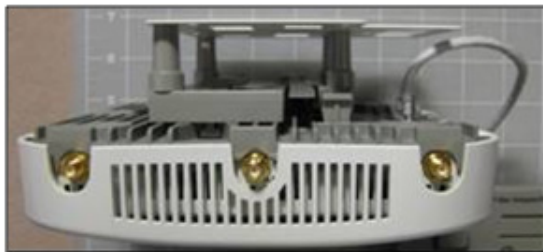
Figure 8: Successful installation (with optional spacers)
