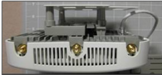
Figure 8: Successful installation (with optional spacers)
