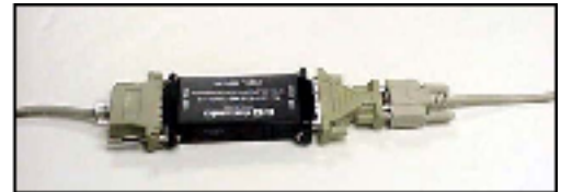
DB9F to DB9M-DB9F Converter
