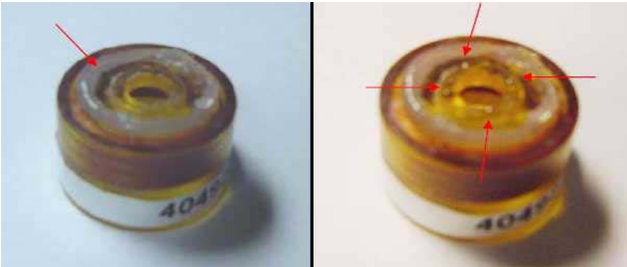
Figure 9: RTV Adhesive ring on the bottom of the case (left); drops of super glue on the inner elevated ring (right).
