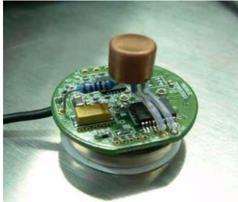
Figure 8: Sensor assembly with sensing element within copper enclosure.
