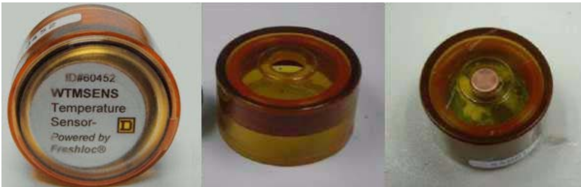
Figure 7: The sensor: the top of the sensor with RFID label seen through the transparent lid and the label attached to the side of the case (left), the empty case of the sensor bottom up (center), the bottom of the assembled sensor with the sensing element in copper enclosure inserted into the opening in the bottom of the case (right).
