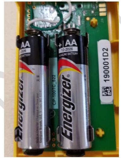
After replacing the batteries, place the front and rear faceplates back together, replace the screw and hold button for < 3 seconds.
