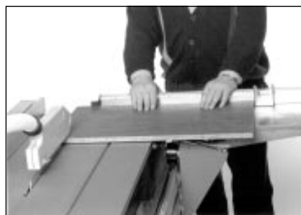
Pull sliding carriage back. Turn work around by 180°, swing flipstop down again and place squared edge against the stop. Make second cut.
