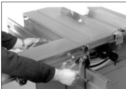
Place table onto traversing saddle and secure with locking levers.
