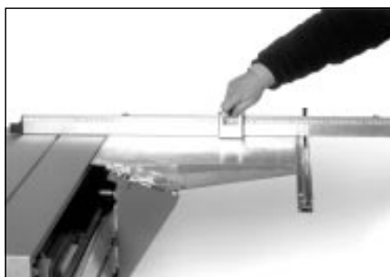
Use tape or stick measure to set flipstop to desired width.
