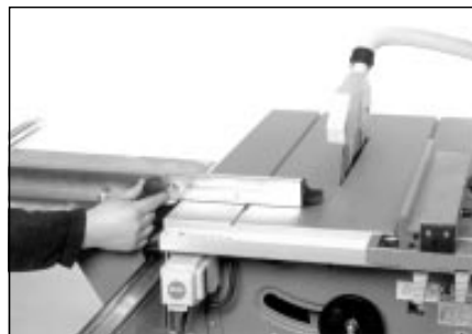
Set fence extrusion closely against the blade, tighten knobs.
