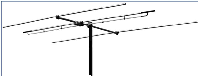
The information bandwidth of the system is less than 25 kHz, therefore, a very narrow bandwidth antenna may be used when operating on a single frequency. In a two-frequency network the bandwidth of the antenna must be wide enough to accommodate both frequencies. The antenna must provide a 50 ohm load. In the U.S. CONUS Network, two frequencies are used: TX = 45.90 MHz and RX = 44.20 MHz. The Bandwidth of the antenna used is 1.7 MHz.
