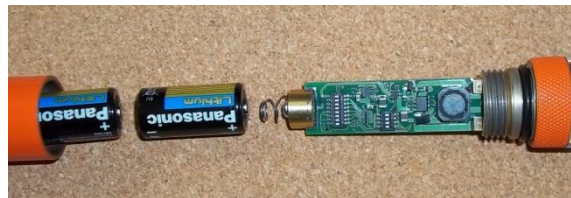
Figure 4: PCB removed for battery change
