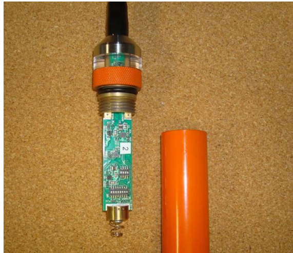
Figure 2: PCB Removed From Pressure Case
