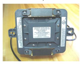
2] Remove the battery pack from the bottom of the CTM enclosure and disconnect the battery pack connector.
