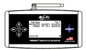
To look at the detailed information that is sent from the Satellite Repeater, push the up and down arrows until the selection arrow is pointed at the entry for the Satellite Repeater. Then press the right button.
