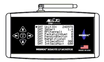
Screen five shows information about the Axonn® STX-2 Globalstar® Satellite Transmitter module.
