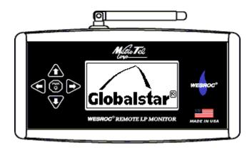
To view Wesroc® RMS transmitters, press the right button from the logo screen. When power is applied to the Satellite Repeater it will transmit status information. The transmitter list screen shows which transmitters have been heard from. The Serial Number of the device, the type of device, the Time Since Last Transmission and the Received Signal Strength are shown. The transmitter screen will look something like this:
