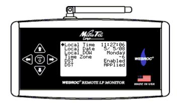
Screen three shows local time information. This information is derived from Universal Coordinated Time as obtained by the Global Positioning System receiver. This information will not be valid until the Satellite Repeater's GPS receiver has obtained a good position fix. Screen three shows:
