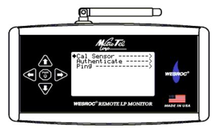
NOTE: A PDU with firmware earlier than version 5.0 will not have a Command List Screen, but will instead show the 'Ping' command on the Main Menu Screen. The firmware on most PDUs can be updated to include the Command List Screen. Check with WESROC Monitoring Solutions customer support for assistance.
