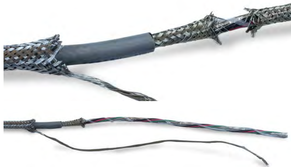
Figure 2-37: Removing the Inner Braided Shield
