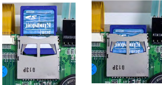
Figure 2-70: Sliding an SD Card into the SD Socket (left); SD Card Installed (right)
