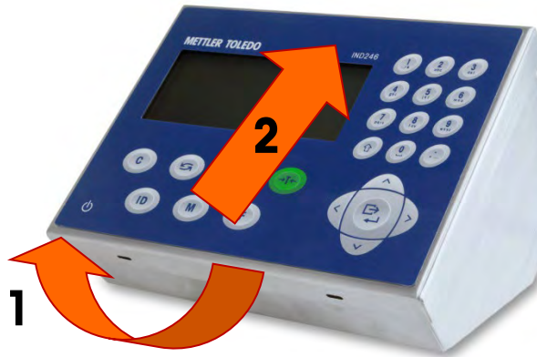
Figure 2-2: Removing the Cover
