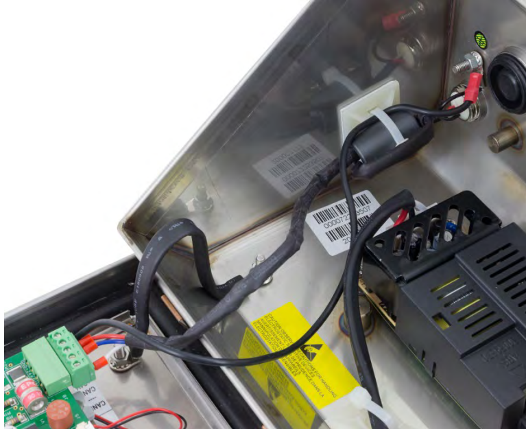
Figure 2-56: PowerDeck Connector Installed in the IND246 POWERCELL
