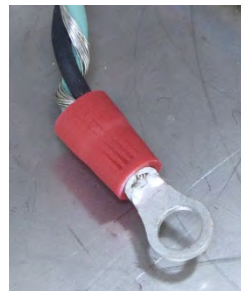
Figure 2-53: Ground Wire Termination
