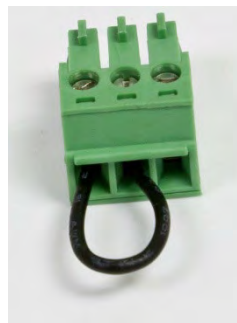
Figure 6-6: Jumper Wire Between COM1 Transmit and Receive Terminals
