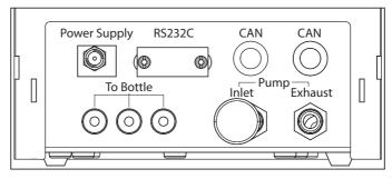
The thinner tube is used for transporting liquid from the bottle to the liquid dosing head. The slightly bigger tube is used for pumping air into the bottle. By adding air, pressure rises in the bottle. When pressure reaches min. 0.3 to max 0.5 bar (4.4 to 7.2 psi) the micro dispensing valve in the dosing head opens and liquid can ascend the liquid tube. The two tubes are further referred to as liquid tube and air tube.
