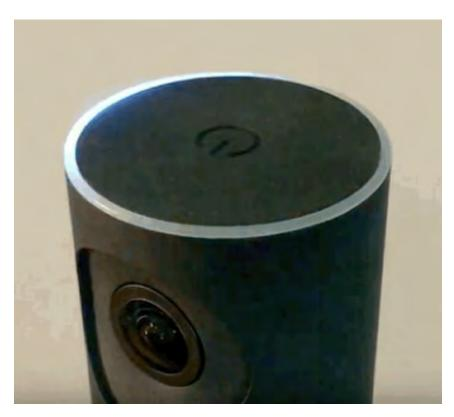
When you are finished using your Mevo, simply press and hold the top button until the LED ring's white light completes a circle around the edge of the camera.
