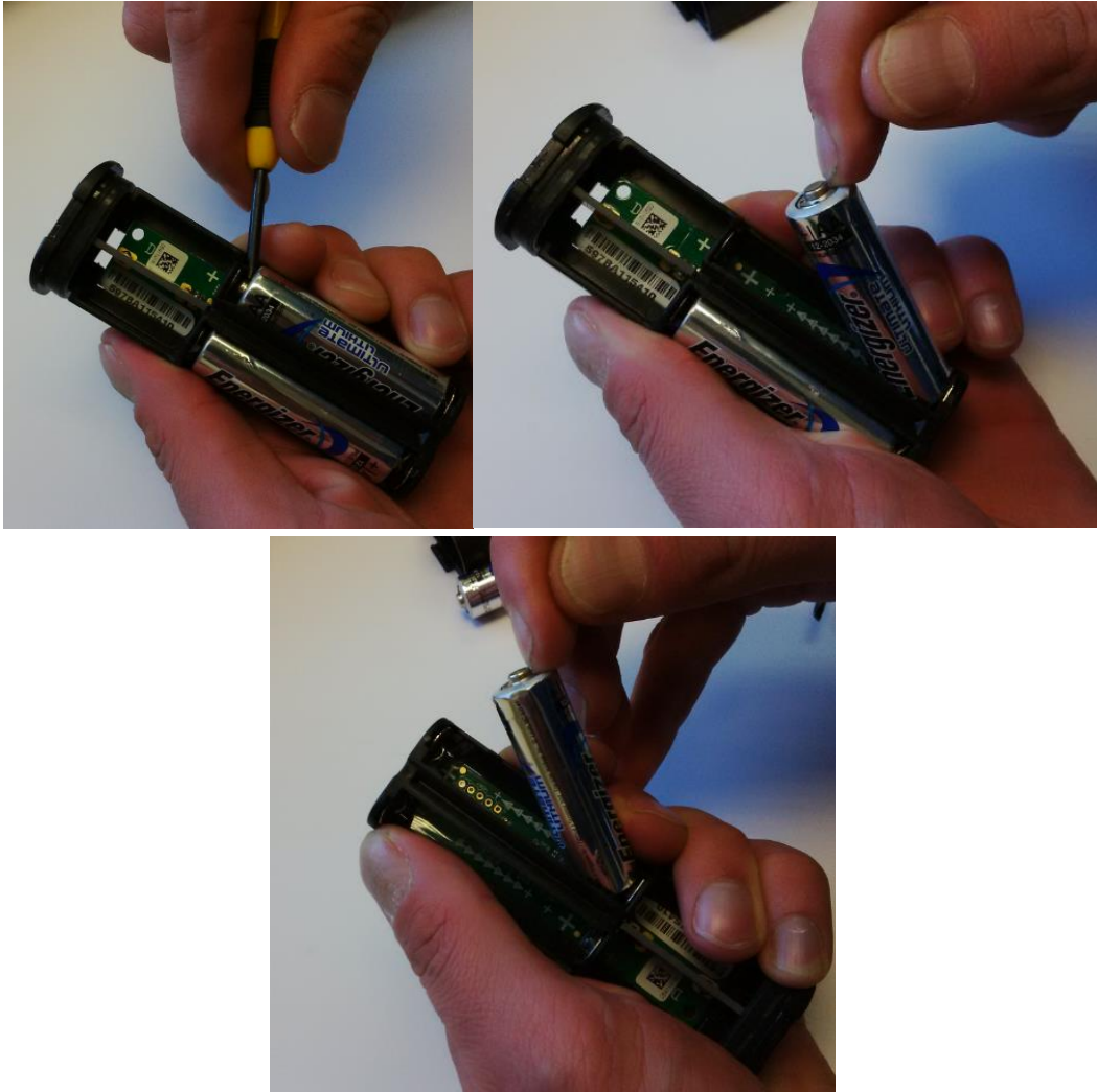
Figure 11 Remove old batteries
