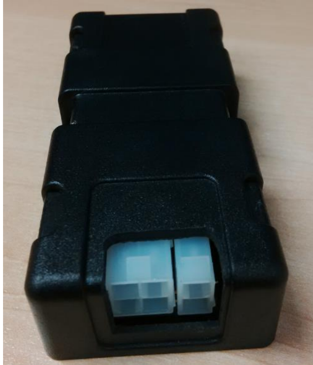
Figure 2–Picture of the Pico Base Station (PBS)
