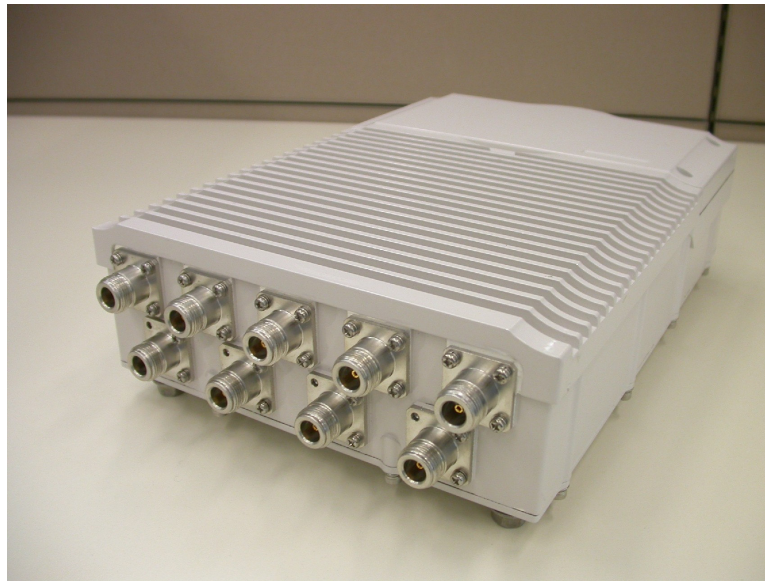
Figure 6. A8 BTS with 802.11a bridge hardware – “a” port
