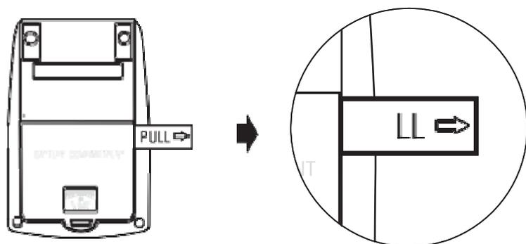
1) **Set the year** – Upon removing the protective strip or installing new batteries, the Year number flashes in the display. Use the M Button to select the Year. Press the ON/OFF Button to confirm your selection.
