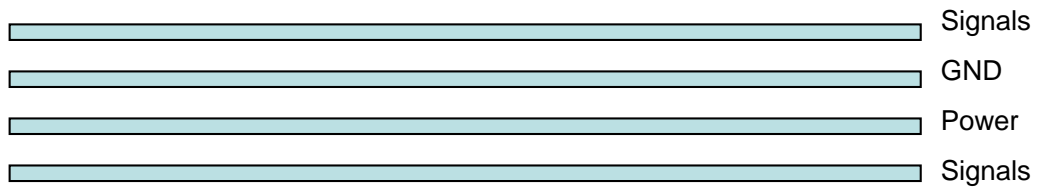
Figure 30: Typical 4-layer PCB construction
