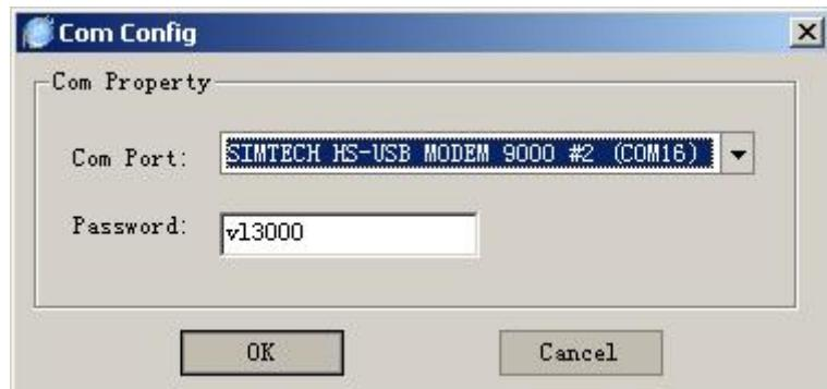
Select the correct com port from the port list, which is displayed in user PC's "Device Manager" and input the password, with the default value "VL3000".
