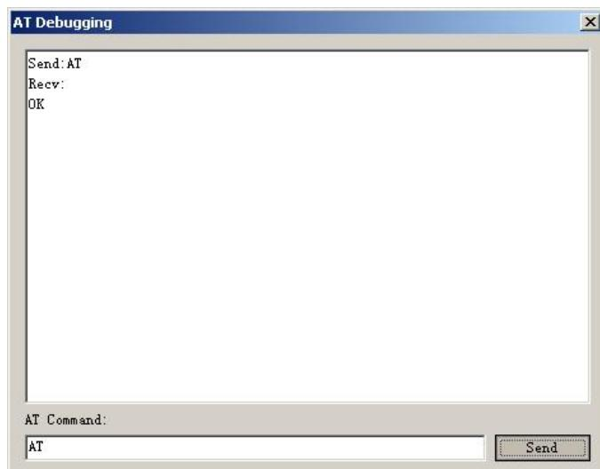
User can test AT command through this window.
