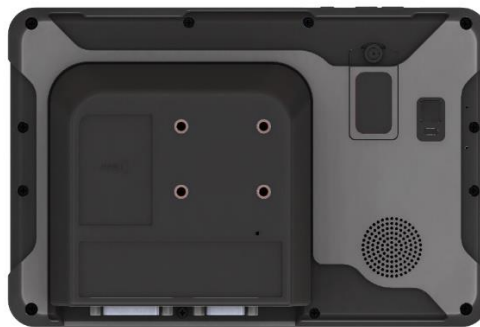
Figure 14: Micronet SmarTab 8 Enhanced Cradle Rear Panel Mounting Arm Screw Inserts
