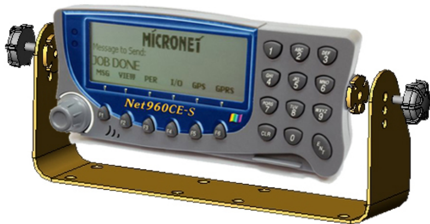
Figure 6: Mechanical Installation – Standard Model
