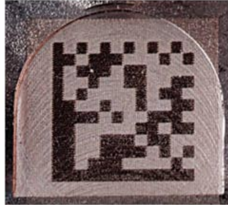
This close-up of a laser-marked symbol clearly shows the L-shaped "finder pattern" running along the bottom and left-hand sides of the code, with the "clocking pattern" running along the top and on the right. Photo courtesy Microscan Corp.
