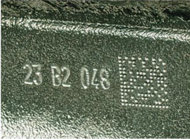
Although dot-peen codes are possible on rough surfaces, engineers should make sure the background texture won't be confused with the actual symbol. Photo courtesy Technifor Inc.
