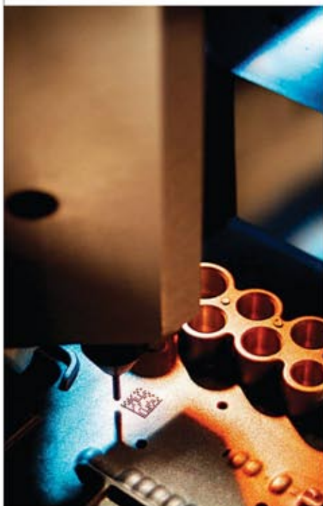
Dot-peen markers can be used to imprint 2D codes on a variety of substrates, including metal. Photo courtesy Columbia Marking Tools Inc.
