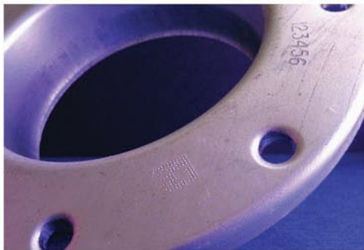
It pays to think ahead about a particular application's part marking requirements, because not all components have as much symbol space as this one. Photo courtesy Pannier Corp.
