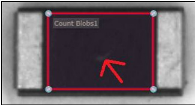
Count Tool (Blob Count) struggling to detect a subtle scratch on part.
