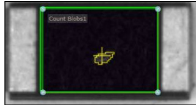
Count Tool (Blob Count) with Gradient Image (Sobel) enabled, Light Pixels.
