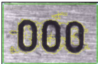
Count Tool (Blob Count) struggling to count features on a metallic surface.
