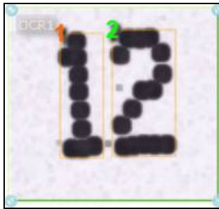
OCR with Grow Objects (Dilate) enabled, Dark Pixels, 1 Iteration.
