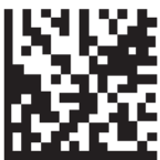
Figure 1: A Data Matrix symbol. The solid black lines on two axes help readers locate and properly decode the symbol.
