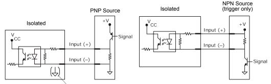
New master pin input (-) is internally grounded.
