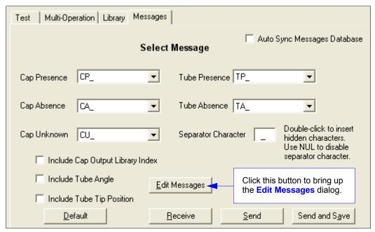
**Note:** The functions in the above view can also be set using the **<K850>** and **<K851>** serial commands.
