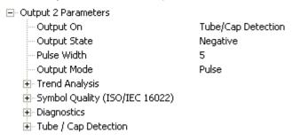
Serial Cmd: <K811,output on,output state,pulse width,output mode>
