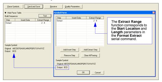
You can extract and insert several character sequences using **ESP**'s **Symbol Parse** feature. In this example, the selected extraction range is characters 2-4. The "Sample Symbol" example on the **Symbol Parse** dialog shows the selected character positions extracted and output as desired. Simultaneously, the data string from the actual selected symbol is displayed at the bottom left of the **Parse Table**, followed by the user-defined extracted output.
