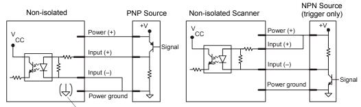
New master pin input (–) is internally grounded.
