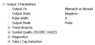
Serial Cmd: <K812,output on,output state,pulse width,output mode>
