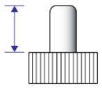
Definition: The length of the cap tip (millimeters/10).
