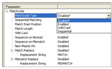
Serial Cmd: <K223,matchcode type,sequential matching,match start position,
