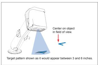
**Important:** The entire object of interest (tube, cap, or symbol) should fall within the field of view (FOV) of the imager. The field of view is what appears in **ESP**'s **Locate/Calibrate** window in **EZ Mode**.
