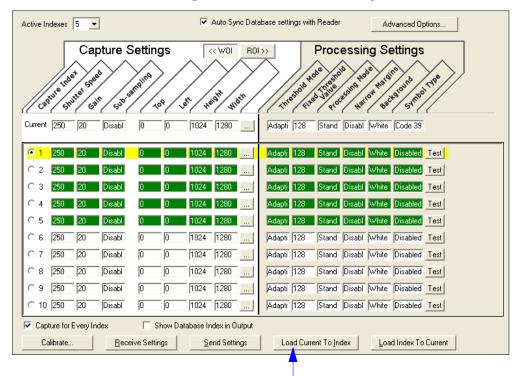
Click the **Load Current to Index** button to save the imager's current configuration parameters to the selected database index.
