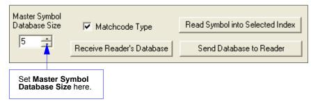
**Caution:** Since the total number of characters available for the master symbol database is **3000**, changes to the **Master Symbol Database Size** will re-allocate the number of characters available for each master symbol and could cause existing master symbols to be deleted (except master symbol #1, unless it also exceeds the size limitation).
