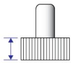
Definition: The length of the cap base (millimeters/10).
