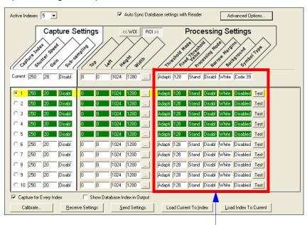
Threshold Mode, Fixed Threshold Value, Processing Mode, Narrow Margins, Background, and Code Type are all Processing Settings values.
