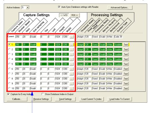
Camera settings (Capture Index, Shutter Speed, Gain, Sub-Sampling) located in the left half of the highlighted area.
