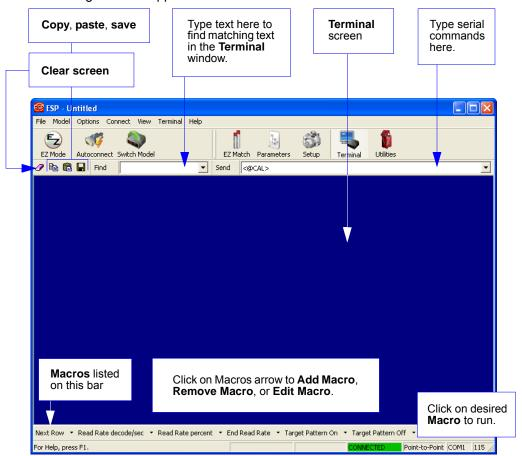
The **Terminal** screen allows you to send serial commands to the imager by using Macros, by copying and pasting, or by typing commands in the **Send** text field.
