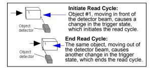
Usage: This mode is effective in an application where the speeds of the conveying
