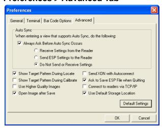
The **Auto Sync** options at the top of the **Advanced** tab allow you to determine whether Auto Sync will be enabled automatically in sections of **ESP** where it is used, or if it will ask you before it enables Auto Sync functions.
