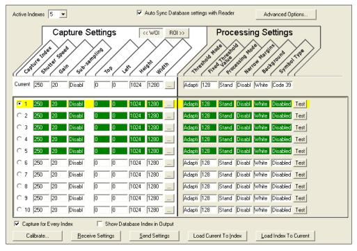
IP Database view, set for 5 Active Indexes, with Capture Settings highlighted
