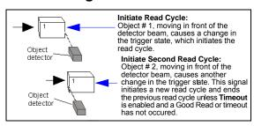
Usage: This mode is highly recommended in any application where conveying
