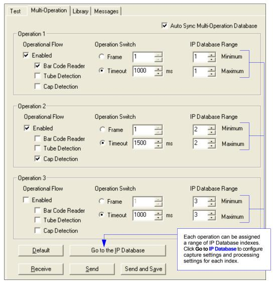
Note: All functions in the above view can be set using the Multi-Operation serial command <K260>.
