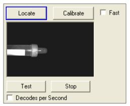
The object in the field of view will appear in the video view beneath the **Locate** and **Calibrate** buttons, and you will see the blue target pattern projected from the front of the imager.
