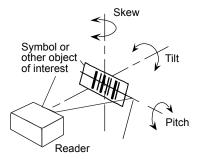
Objects can be rotated at any angle; however, for best results, objects should be aligned with the FOV (field of view).
