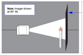
Place a black background behind the area where test tubes, caps, or symbols will be inspected by the imager. This is important because it provides the contrast necessary for the imager to detect the presence or absence of objects in the field of view.
