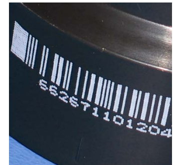
Some DPM marks can be decoded with a laser scanner
