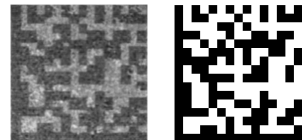
Comparison of direct part mark and Data Matrix after processing
